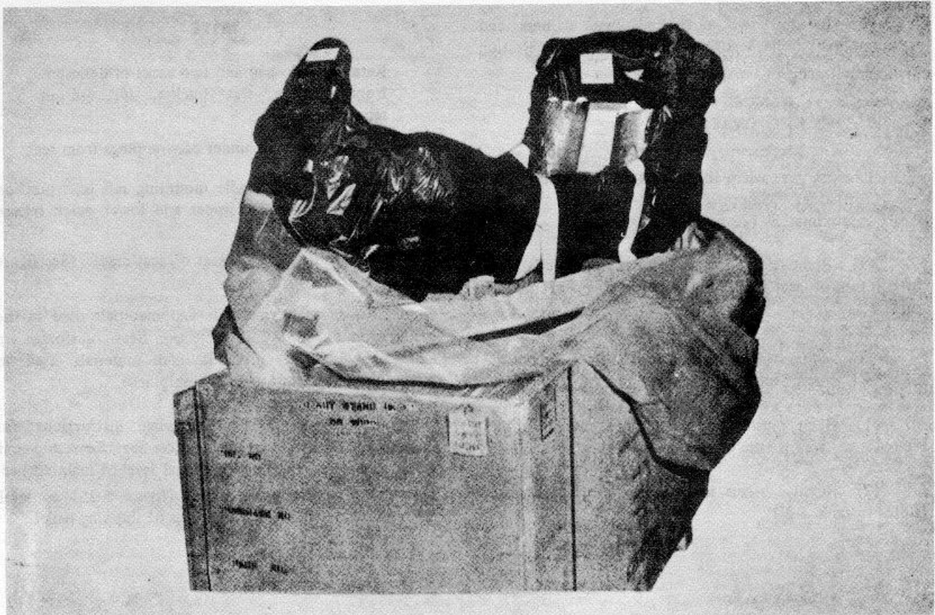
Figure 5-24. Ejection seat with outer wrapping removed
